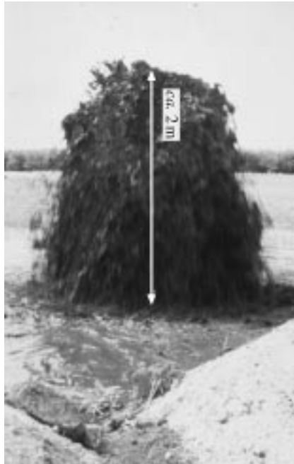
Figure 3. Eruption of pore water after an underground explosion.
